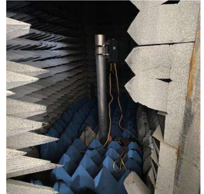
RF Anechoic Chambers for antenna characterisation
