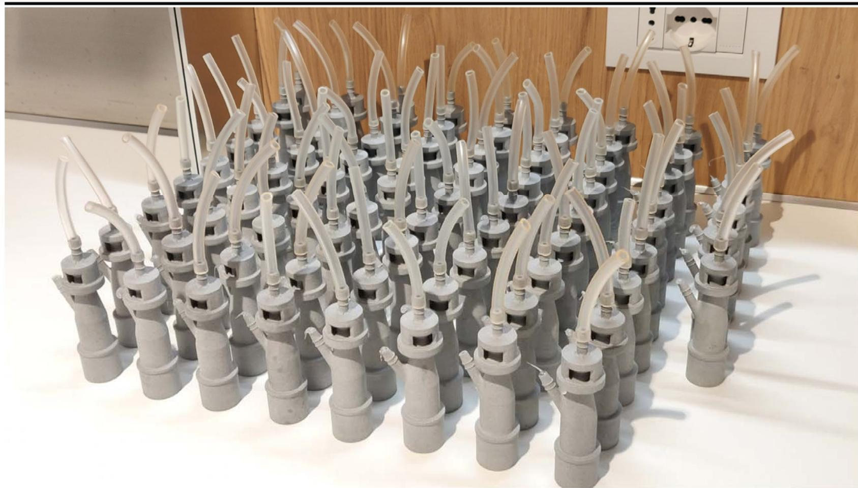
*3D printers fabricate emergency valves for ventilators to keep coronavirus patients breathing*
